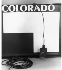
• When a fingertip is pressed against the surface of the touchpad, the entire red bar graph should illuminate; if it does not, you have an open touchpad (a touchpad that will not send a signal). Contact CTS customer support.
